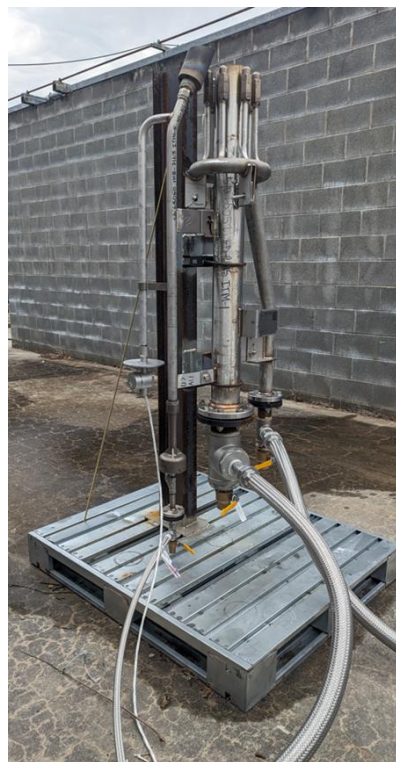
Figure 1: Picture of the Georgia Tech gas flare test rig. The air-assisted flare tip was manufactured by Zeeco.
