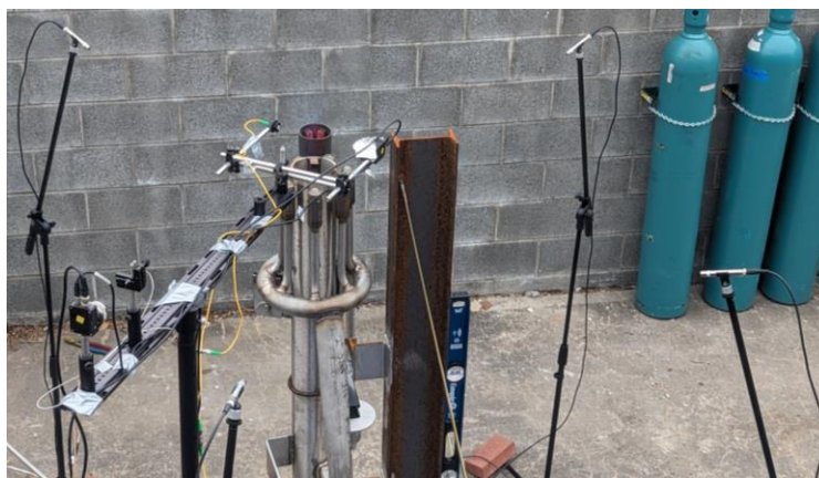
Figure 2: Setup of sensors for acoustic and absorption spectroscopy measurements in the Georgia Tech flare test rig.
